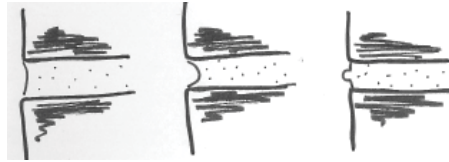
Good examples of pointing - from left: flush, smooth and tuck pointing
