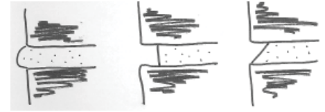
Bad examples of pointing - from left: exposed, weather-struck and weathered pointing
