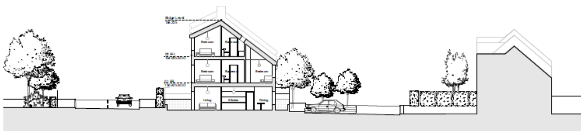
Image 9 – Section of proposal including proposed retaining walls.
