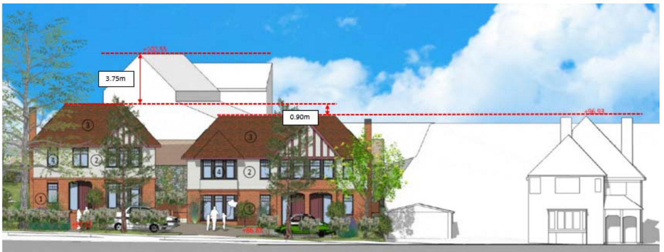
Figure 6-Height Differences Between Site and Neighbouring Properties (officer's measurements and markings)
