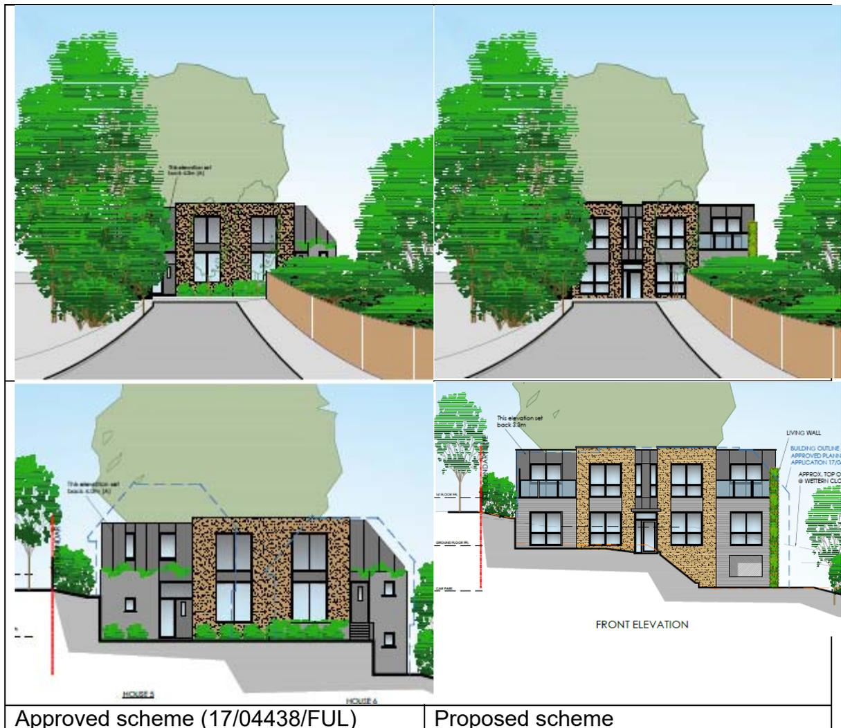
Figure 4: Front elevations showing changes at the rear between the approved and proposed schemes
