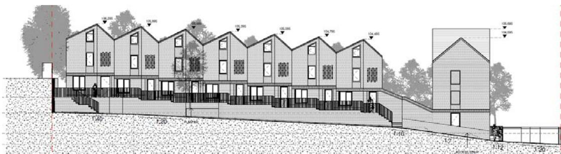
Figure 4 Front elevation of terrace showing levels and retaining wall
