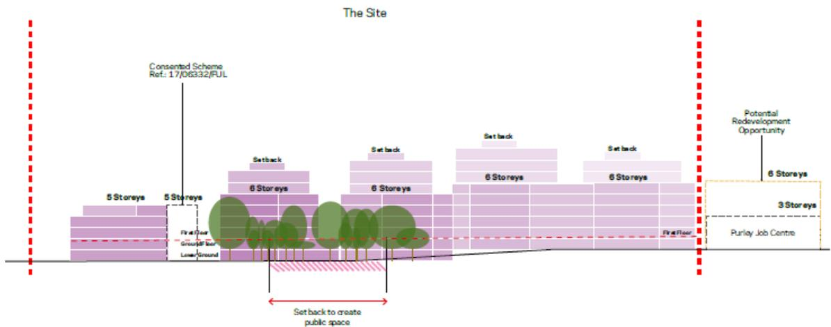
Fig 8 – Massing Section of front elevation showing land level changes and relative floors.
