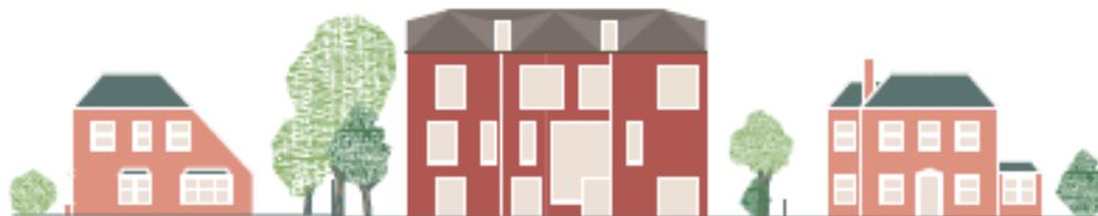
Figure 2.10c: Where surrounding buildings are predominantly detached dwellings of two (2) or more storeys, new developments may be three (3) storeys with an additional floor contained within the roof space or set back from the building envelope below.
