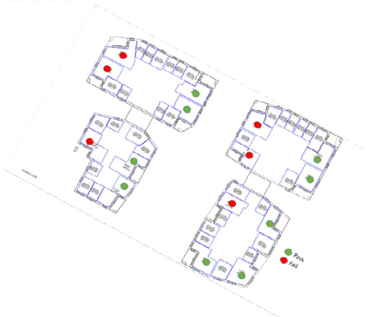
Fig 7 - Showing location of sunlight BRE pass/fails at second floor level
